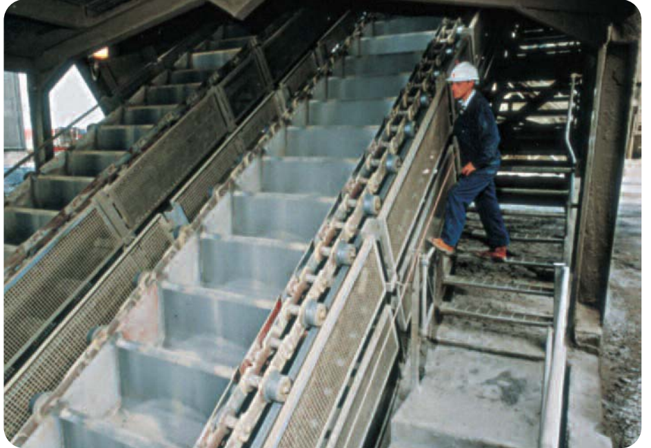
特殊双股输送链设计能够延长链条在水泥炼砖这样高温和高尘环境中的寿命。 Special Double Strand Conveyor Chain is designed to give an enhanced chain life in the hot and dusty conditions of a Cement Clinker.
